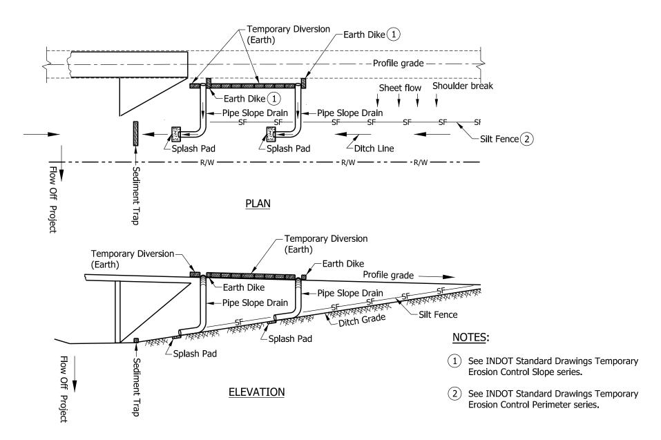
UNDISTURBED SIDE DITCH TREATMENT
